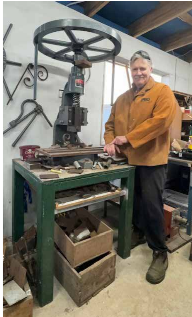
Moi cold forming scroll with a flypress imported from India – one of the few places still making this tool.
